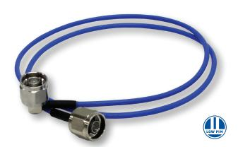
Microlab Model JB series, Coaxial Jumper Cables are built for reliability and consistent extremely low PIM performance. Designed for use in all systems where low PIM and very good R.F. and mechanical performance is critical. Using controlled manufacture, low PIM cable and trimetal plating the connectors ensures good intermodulation performance.
