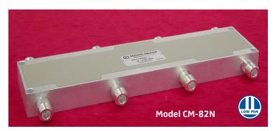
This broadband 4:2 Hybrid Combiner is a network of three couplers in a convenient package with high isolation in the wireless bands and low passive intermodulation (PIM). Four inputs feed two 3 dB hybrids whose outputs are fed to a third 3 dB hybrid coupler.
