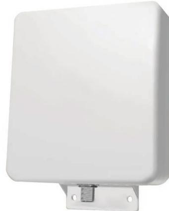
The YA-20NF is an attractive Low PIM Directional antenna. These antennas are popular for propagating wireless signals in distributed antenna systems, (DAS). This wideband antenna covers all common wireless and WiFi bands in the range of 698 to 6000 MHz such as 700, 800, 850, 900, 1700, 1800, 1900, 2100, 2400, and 2600. This model is weather resistant.
