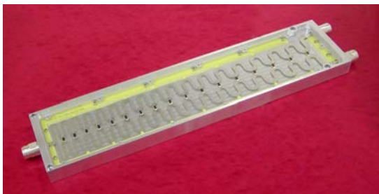
Fig 4 Ultra wideband 70 to 2700 MHz Wilkinson Divider/Combiner using 17 sections with an air dielectric for minimum loss
