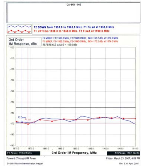
Fig 17 Actual PIM performance of a Wideband Hybrid Coupler
