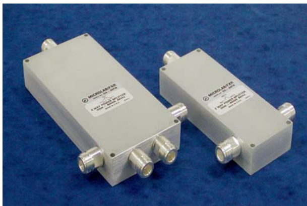
Fig 5 From UHF to WiMAX 350 to 6000 MHz Wilkinson Divider/Combiners in 2 and 4 ways using a microstrip design
