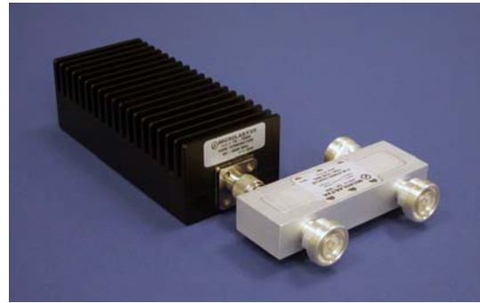
Fig 3 High Power Hybrid Combiner with 100W load for base station combining
