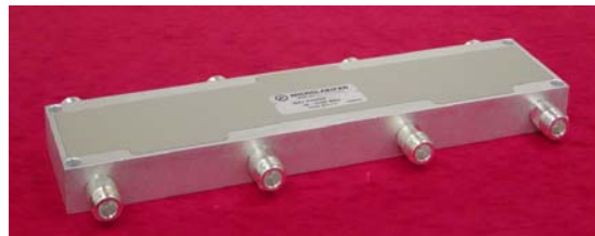
Fig 9 Simple 4 input 2 output multi-band 700 – 2700 MHz Combining Matrix using three Hybrid Couplers and two external loads
