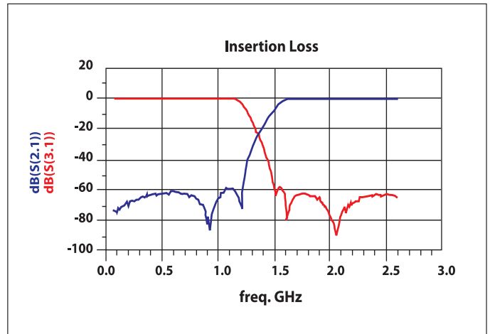
Fig 3: Insertion loss characteristics of a Microlab diplexer
