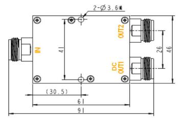
Microlab Model D2-79FN Wilkinson style 2 way Power Divider is based on the D2-69FN. It has been designed for GPS applications, which require only one signal path to pass DC. The unit has broad frequency coverage from 694 to 2700 MHz, and offers high output isolation and good VSWR.
